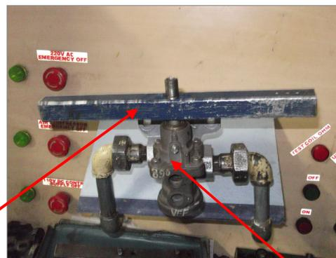
Fabricated tool for armature removing
